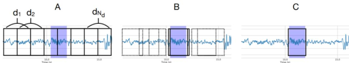
Prediction procedure for DOSED. A:  $N_d$  default events  $d_i$  are generated over the EEG sample. B: network predicts potential events (adjusted centers and durations, potential event labels). C: non-maximum suppression. network returns centers, durations and labels of events (Chambon et al. [2018])
